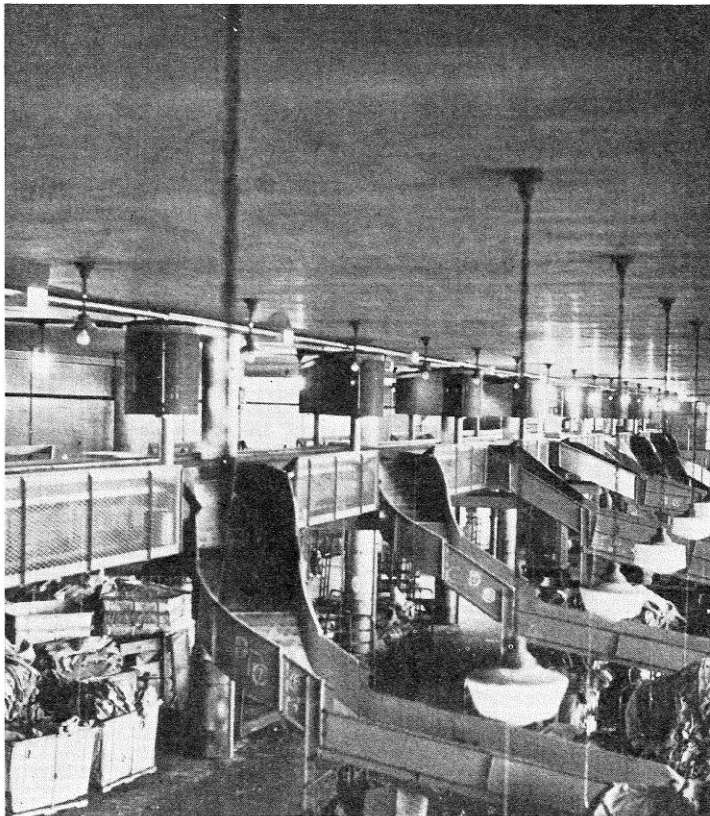
Fig. 10 — Parcel Sorting Machine Using Sweeps for Parcel Diversion — U.S. Post Office.
