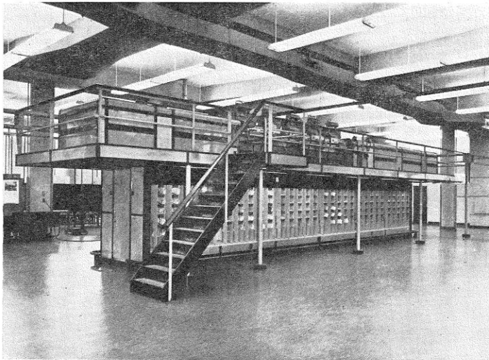
Fig. 3 — Transorma Machine Manufactured in Holland. 5 positions — 300 or more separations. Manual feed to operators — manual clearing.
