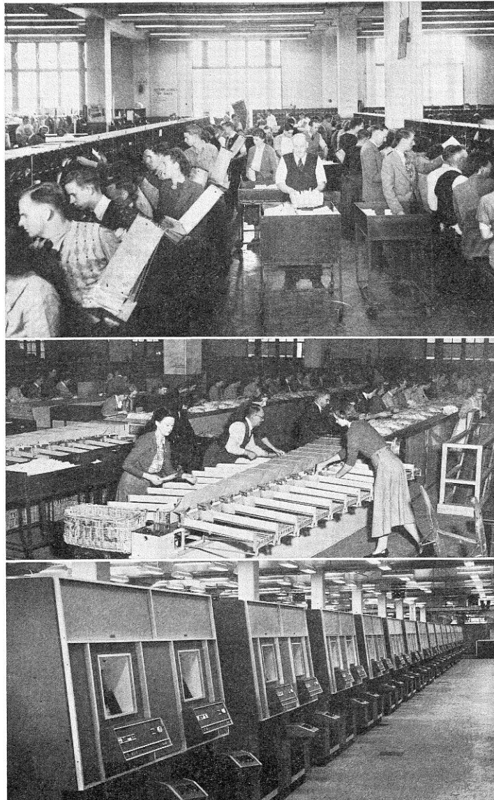
Fig. 4.—Developmental Stages in Letter Processing. Top: Until the year 1960, all letters were primarily sorted on upright presses in all mail exchanges. Middle: Machines designed to aid the sorting and distribution processes and installed to replace upright primaries. Bottom: One of the five suites of coding positions installed in the Sydney Mail Exchange. Letters, when coded, can be processed automatically.
