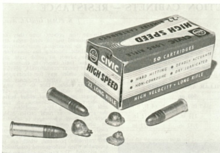
Fig. 2 — Cartridges used in Tests and Examples of Deformed Bullets after Testing.
