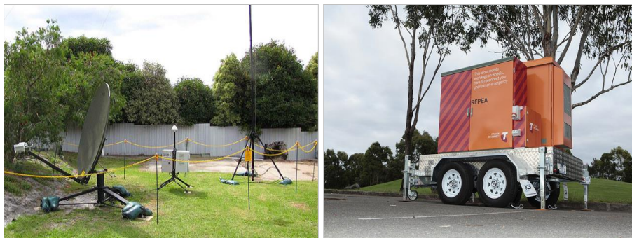
Figure 2 – a) Satellite Cells on Wheels b) Mobile Exchange on Wheels, Source: (Piltz 2013)
