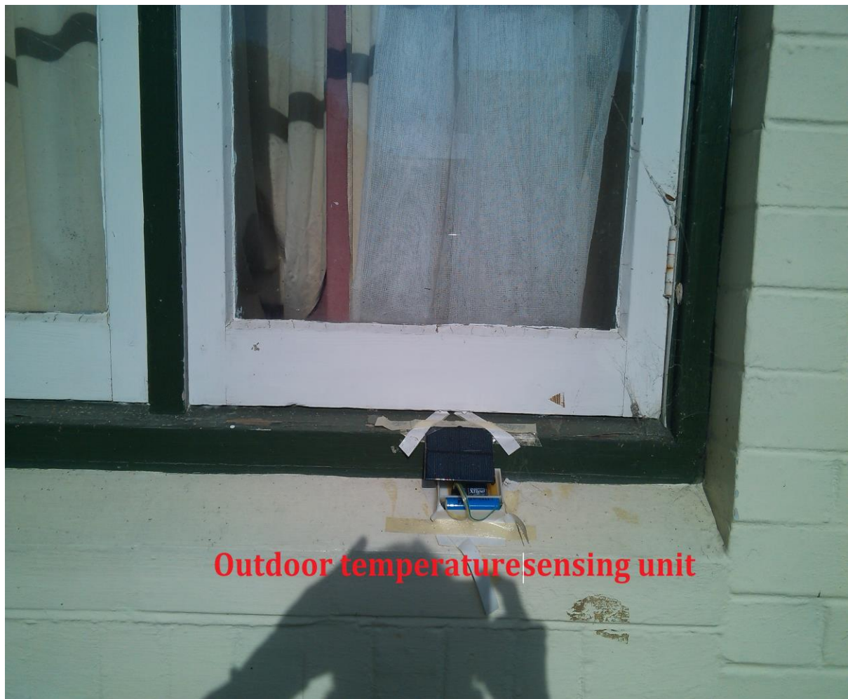
Figure 7. Outdoor sensing unit for outside temperature measurement
