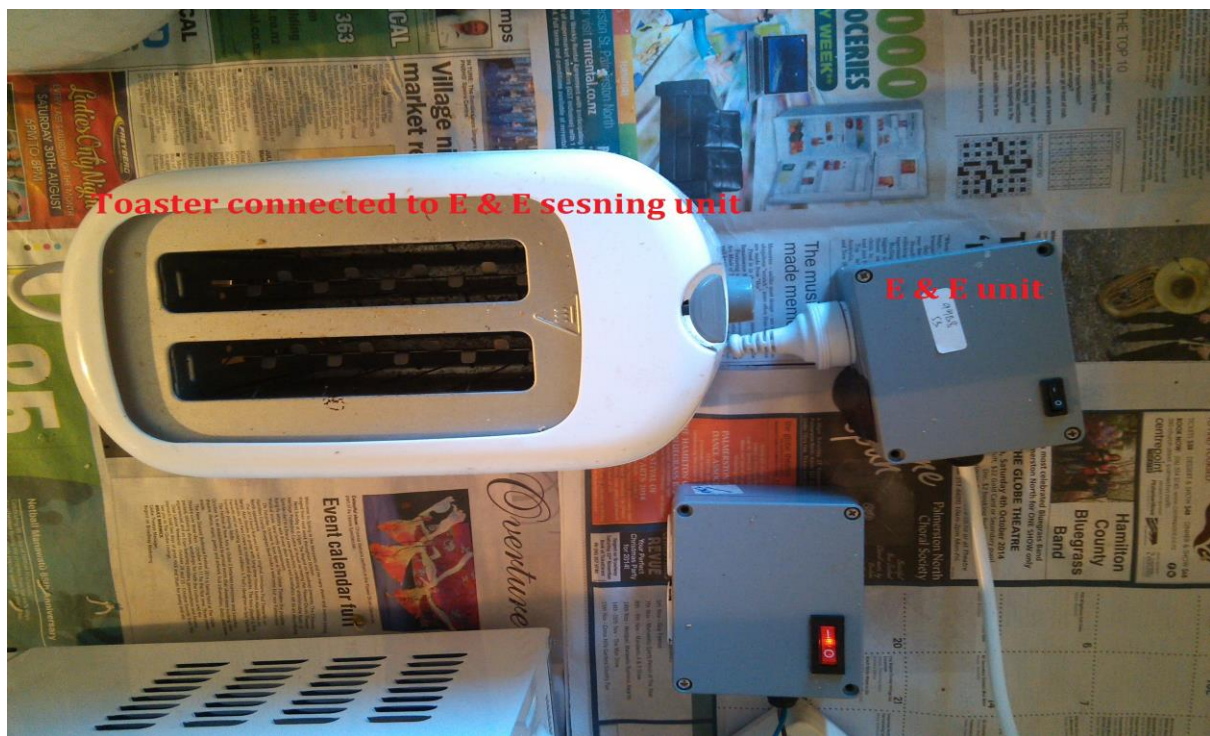
Figure 5. Toaster plugged to wellness protocol based E & E power usage and control unit
