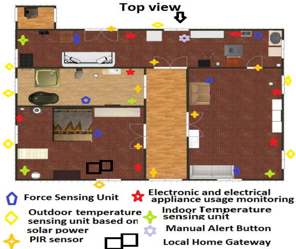
Figure 4. Layout of sensor deployment in the smart home
